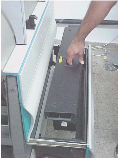
Lifting the unloading/accumulating cassette out of its drawer
