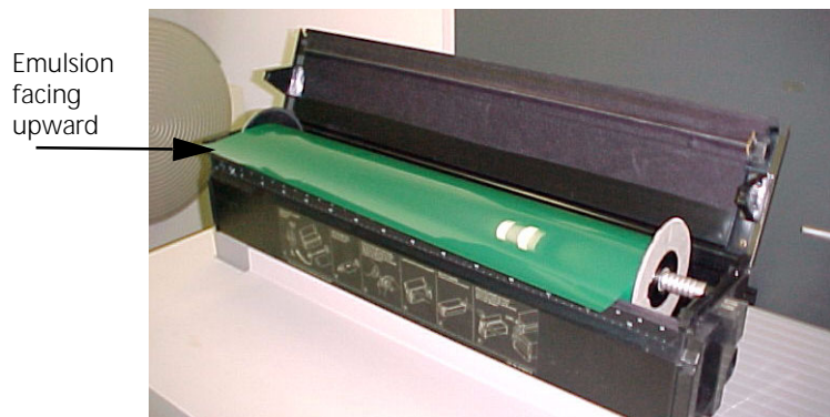
Inserting the film spool into the loading cassette
