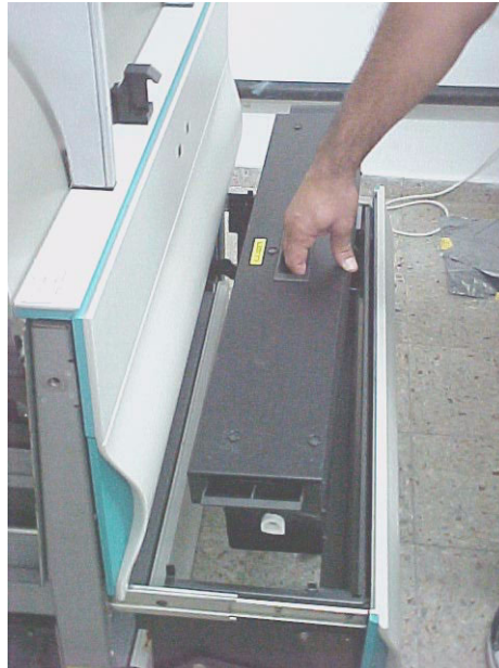
Placing the unloading/accumulating cassette in its drawer
