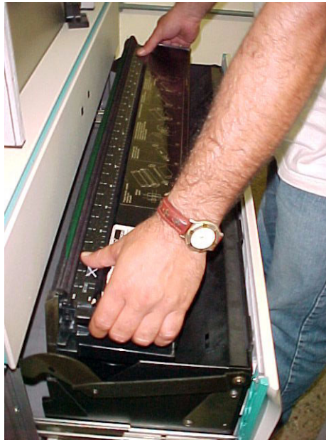
Placing the loading cassette in its drawer
