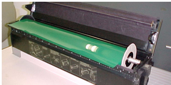
Unloading/accumulating cassette (before flipping around) with film sticking out
