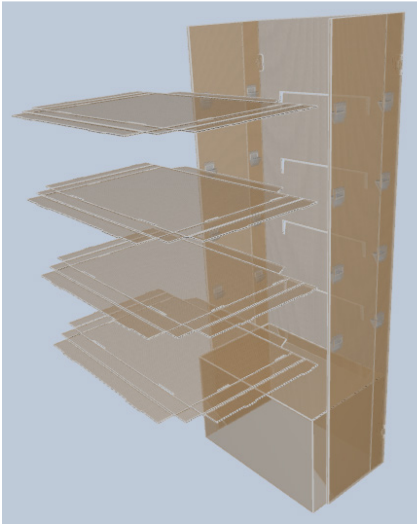
Pic. 59: The four shelves are positioned into place.
